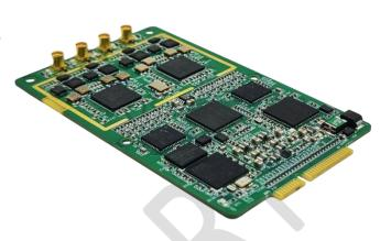
The purpose of using the KV-AJ2.C-OEM module is to ensure stable reception of the navigation signal in conditions of staged interference. The module can be used with the KV-AJA phased antenna array, and can be separately integrated into a third-party device. The product supports the GPS, GLONASS, Galileo, NavIC satellite constellations and can be employed for the land, sea, air platforms (including unmanned aerial systems) and fixed installations.
